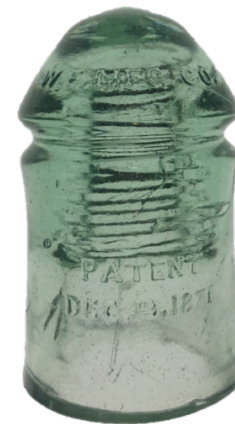
CD 102 Brookfield found on an abandoned telegraph line in the Yukon.
