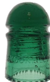
CD 102 Brookfield found on an abandoned telegraph line in the Yukon.
