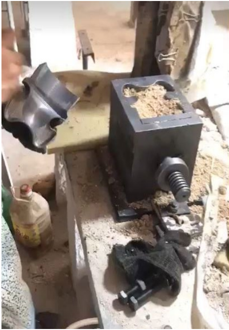
COMPLETED MOLD FILLED WITH THE DRY PROCESS MATERIAL
