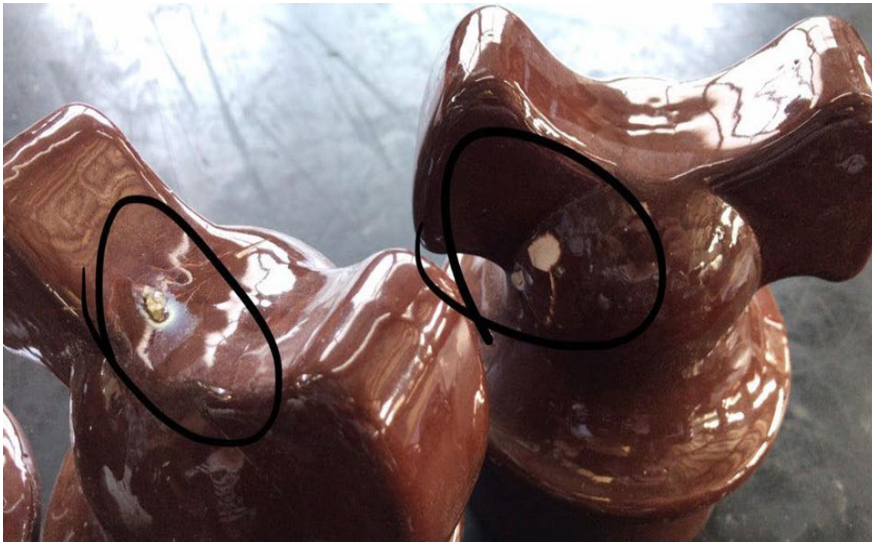
DRY FLASHOVER RATING TEST WHICH WAS 30KV
