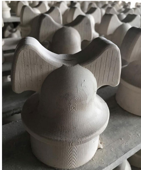
MICKEYS ARE MOLDED AND READY TO BE INSPECTED AND PREPPED
