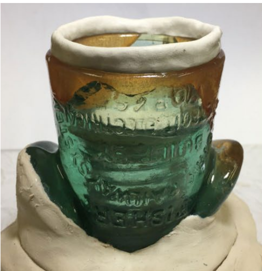
CLAY TO BUILD A POURING CHANNEL
