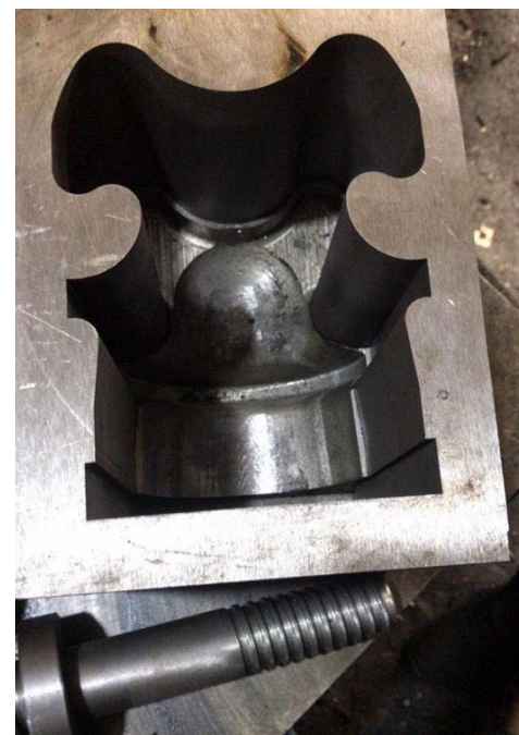
LOOKING DOWN IN THE MOLD BEFORE PIN IS CUT INTO PLACE
