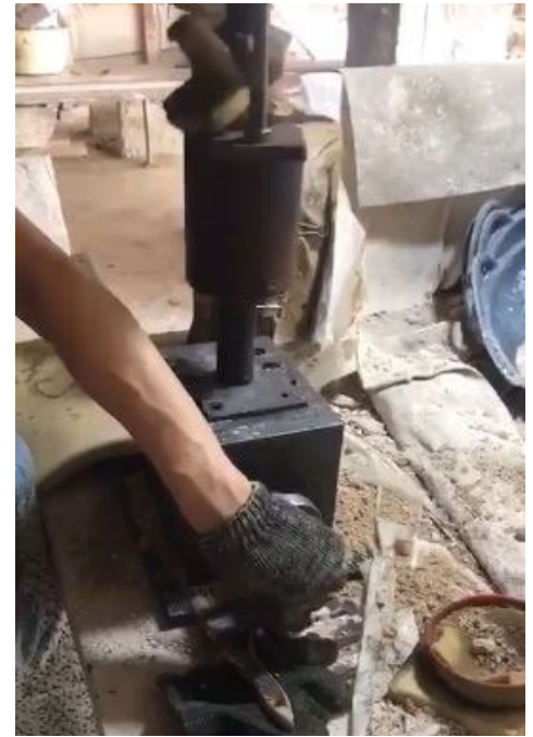
PRESS IS APPLYING PRESSURE TO THE MATERIAL TO FORM MICKEY
