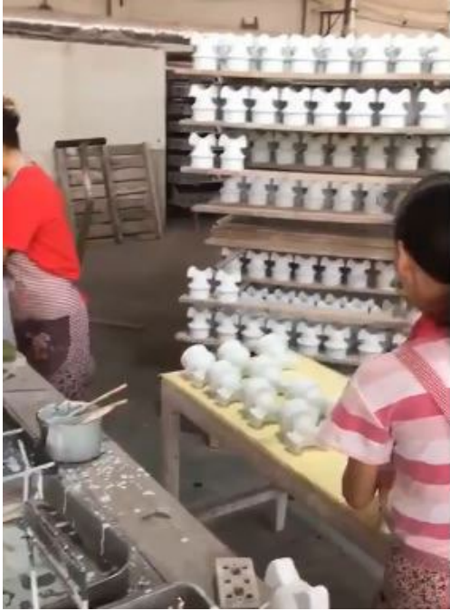
6 MICKEY ARE PUT ON A RACK, DIPPED INTO VAT OF BLUE GLAZE THEN FIRED
