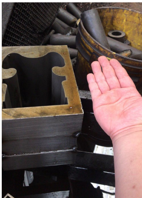
A CLOSEUP OF THE MOLD BEFORE THE BASE PLUG IS CUT INTO IT
