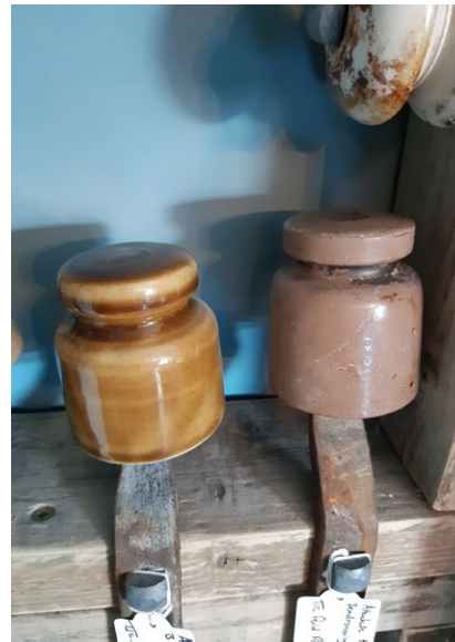
PHOTO 16 – Close up of the Taylor Tunnicliffe field pattern insulators.
