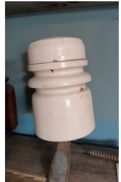
PHOTO 17 - One last unexpected discovery came from the line on a third trip, when we walked a section closer to Attadale house and found a fallen pole with an early large TTC pothead insulator cemented on to the original Curtoys pin!
