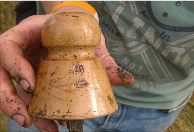
PHOTO 13 – “Stiff London” marked Curtoys just after being rescued from a very rotten pole.
