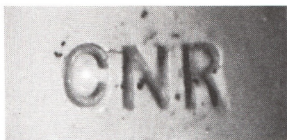
Dry process CNR incuse marking (note the dry process cracks visible through the glaze.)
