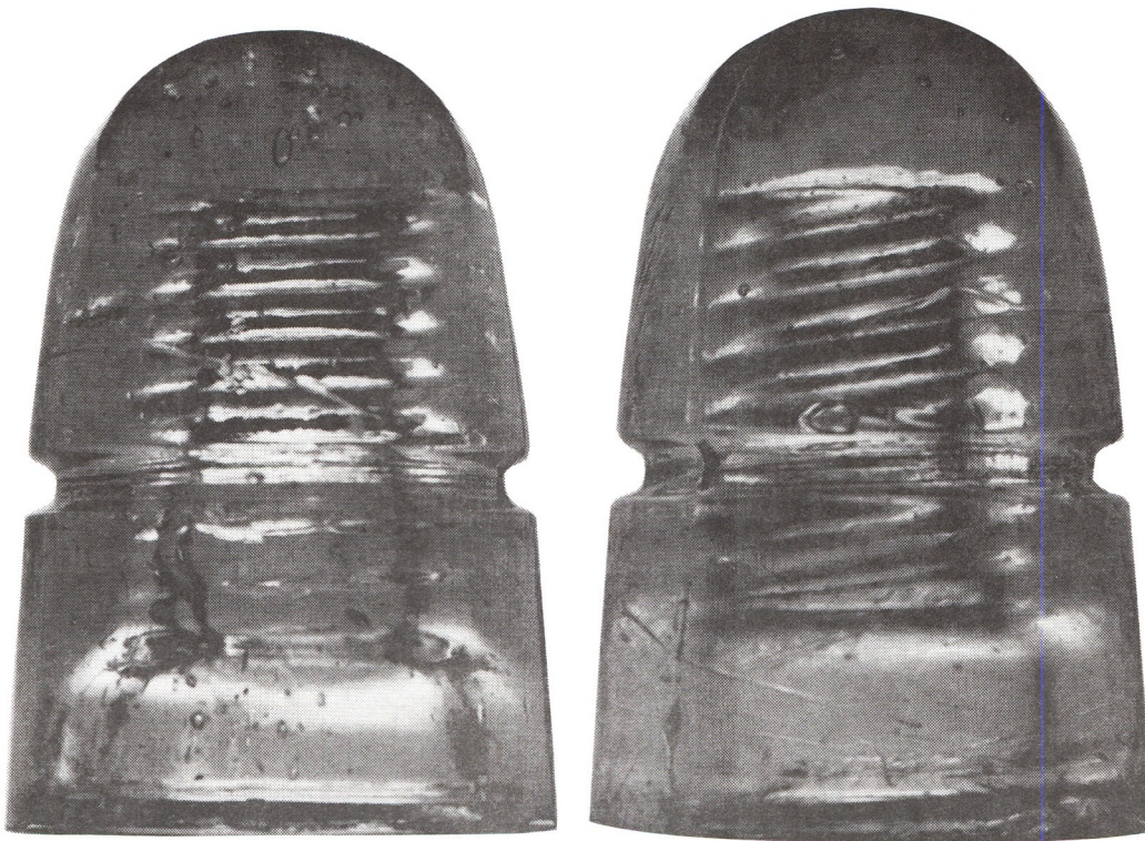
Type 8C single and double-threaded. Note the steeper thread pitch on the double-threaded item on the right.
