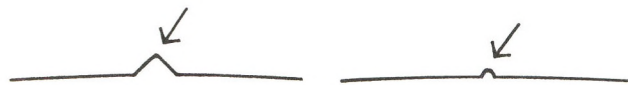
'Chisel point' embossing and regular height embossing. Only the highest areas on the embossings are illustrated.
