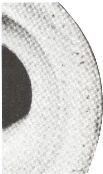
Small crack-like lines in the surface of dry-process items.
