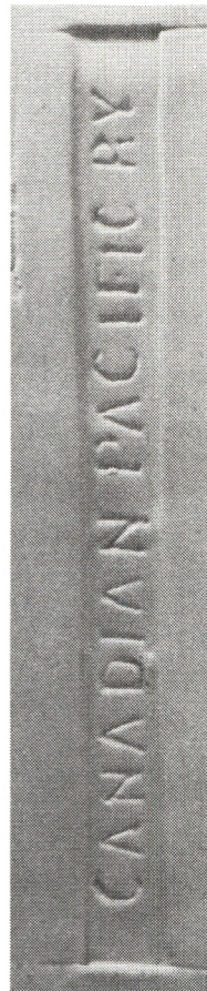
The raised band of the 3C mold style.
