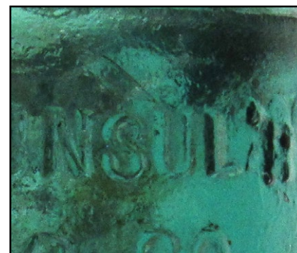
CD 185 JEFFREY MFG. CO. [040] (F-Above wire groove) SPECIAL MINE INSULATOR/JEFFREY MFG.CO. {Many varieties of blot outs and spelling errors at the end of 'INSULATOR'} (F-Skirt) COLUMBUS OHIO/PATENT SEPT 25 1894 {Drip points may be on the top or on the bottom of the insulator} SDP
