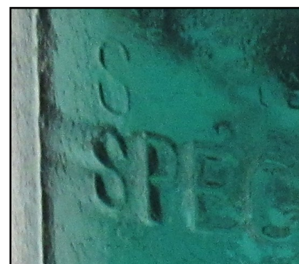
CD 185 JEFFREY MFG. CO. [001] (F-Above wire groove) S/SPECIAL MINE INSULATOR/JEFFREY MFG.CO. (F-Skirt) COLUMBUS OHIO/PATENT SEPT. 25 1894. {Drip points may be on the top or on the bottom of the insulator} SDP
