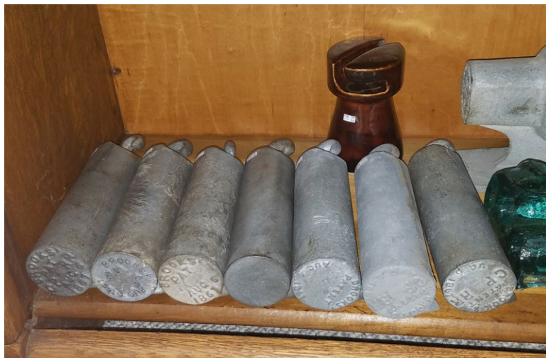
SERIES OF 1867 BROOKS PARAFFIN INSULATORS WHICH HAD A GLASS INSERT AND HOOK. YOU CAN SEE THE ACTUAL INSERT AND HOOK IN THE GLASS HOOK ILLUSTRATION ON THE FAR RIGHT OF THE TOP ROW. ALSO NOTE THE DIFFERENT EMBOSSINGS ON THE BROOKS PARAFFIN INSULATORS.
