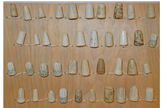
"WIRE NUTS MADE OF PORCELAIN" - DISPLAY BY: RICK SOLLER OF GURNEE, IL (NIA #2958)
