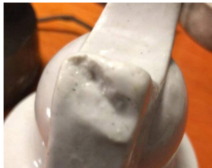
U-379 NN WITH A CHIP GLAZED OVER IN THE FACTORY.
