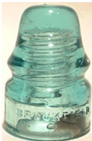
ID 675 - A BROOKFIELD CD 133 WITH A LARGE DIRT FILLED OPEN BUBBLE WITH A VERY TINY OPENING
