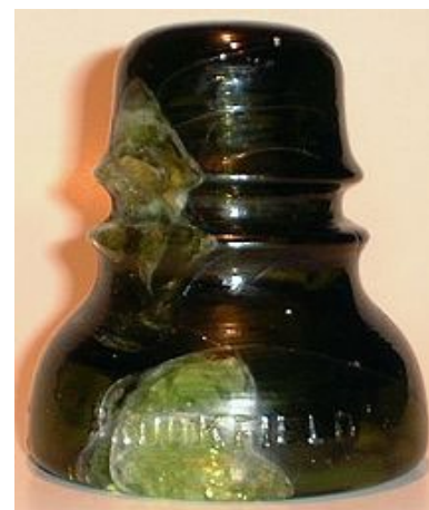
ID 992-A - A BROOKFIELD CD 152 THAT HAS A LIGHTNING FLASHOVER.
