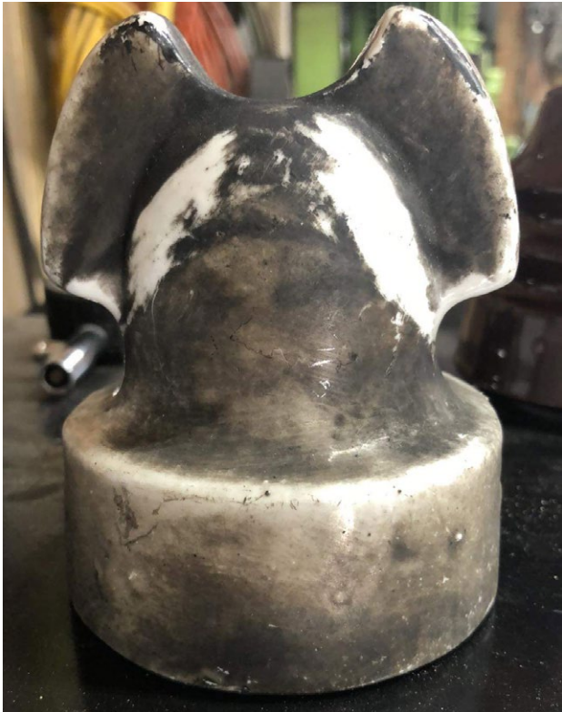
SOOT COVERED U-380
