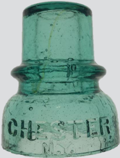
CD 735 Chester. Insulators of this type were widely used on the 1866 section of the Collins Overland Telegraph line.
