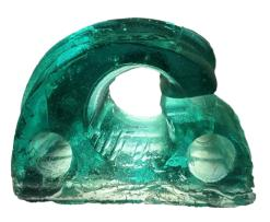
CUTTER WITH WIRE RUBBED GROOVES
