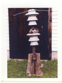
A large multipart rated for 69,000 volts. These were used in the Niagara to Buffalo lines before they were upgraded to suspension insulators. The large head allowed the mounting of substation hardware.
