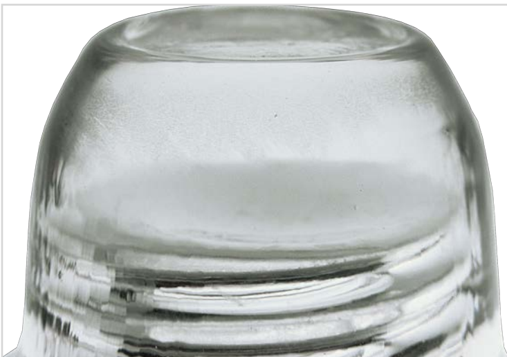
Penny impression in a CDI60 Whitall Tatum. Note poor reproduction of detail, softer edges to impression, and concentric ripples on impressed surface. On the side view note that the dome seems distorted around the impression.
