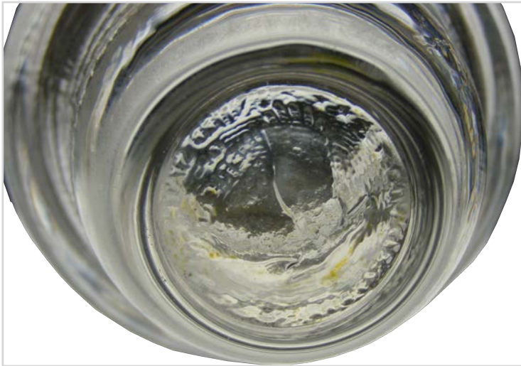
Penny impression in a CDI62 Hemingray 19. Note clear crisp impression, and sharp edges around coin. Also, there is no distortion around the impression
