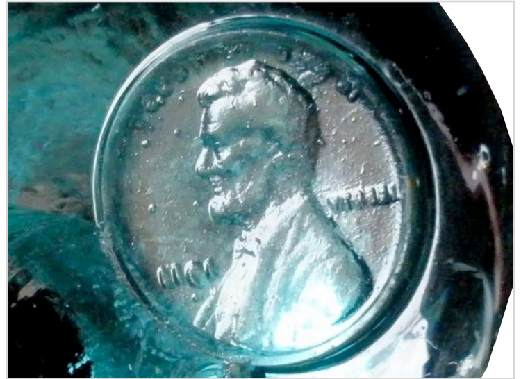
Penny impression in a CDI62 Hemingray 19. Note clear crisp impression, and sharp edges around coin. Also, there is no distortion around the impression
