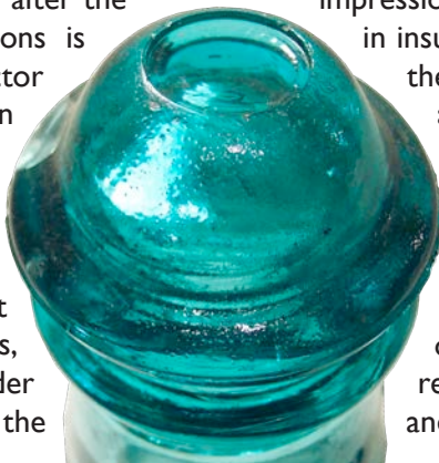
Example of a CD106 that was dug from the Hemingray dump. Note deep and crisp impression with no distortion of the surrounding dome, and consistent glass texture both near the impression and elsewhere
