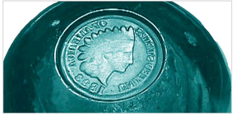
Penny impression in a CDI45 Hemingray-21. Note clear crisp impression, and sharp edges around coin. It is not so apparent from this photo, but there is no distortion around the impression.
