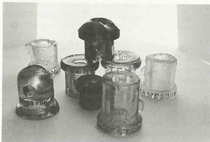
(Figure 1.) A variety of lightning rod insulators. (Collection of Glenn Drummond, photograph by David Dale)
