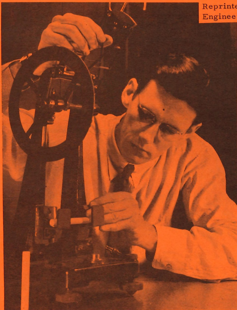
Dr. Russell tests the impact strength of standard and Zircon porcelains. Fore-ground pieces have equal strengths although Zircon specimen is much smaller.
