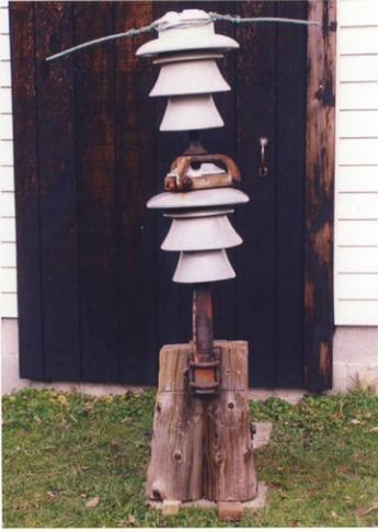
A large multipart rated for 69,000 volts. These were used in the Niagara to Buffalo lines before they were upgraded to suspension insulators. The large head allowed the mounting of substation hardware.
