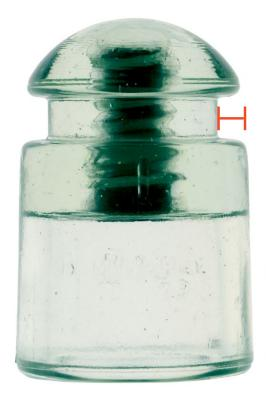
FRONT VIEW OF [080]: WIRE GROOVE APPEARS SHALLOW; VERTICAL BARS ON FRONT & REAR
