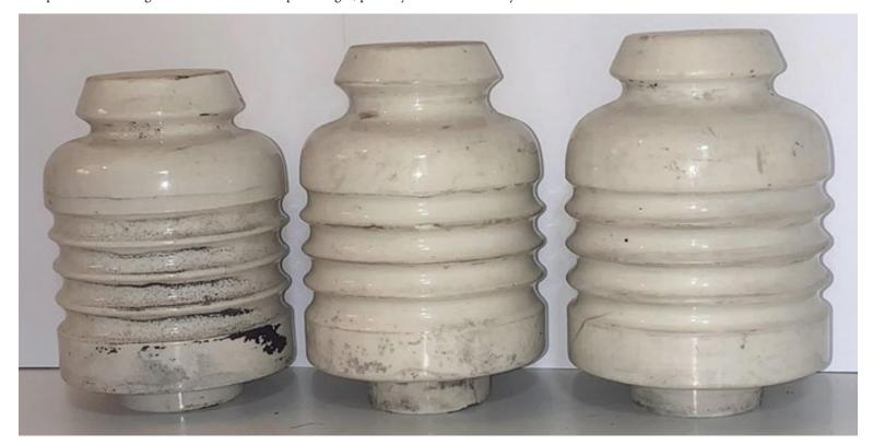
In photo x4, above, you'll see a clear comparison of the different shaped wire grooves on three cream coloured ones. These are stamped FULLER & LANGDON PATENT on the head top.
