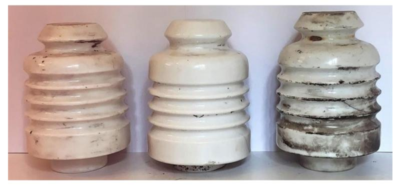
Photo X3, above, shows three examples of these differences on the most common corrugated type, the bright white ones. These are usually unstamped and are thought to have been of European origin, possibly made in Germany or Czechoslovakia.
