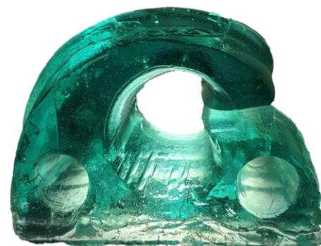
CUTTER WITH WIRE RUBBED GROOVES
