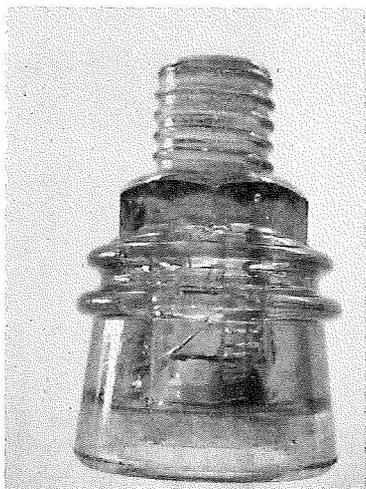
left: CD 458 (aqua) Boston screw top inner skirt embossed BOSTON BOTTLE WORKS PATENT APPLIED FOR from Peg Hotton of Rockville, MD.
